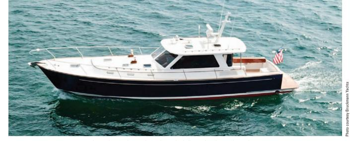
The Bruckmann Abaco 47 has an innovative hull form that planes at just 12 knots.
